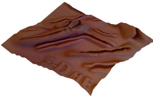
**Fig. 3** 3D model using stereoscopic image-based reconstruction of the original object (Fig. 2)
